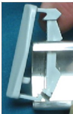
Hook opened to remove retainer
