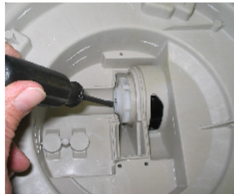
Forcing motor from sump
